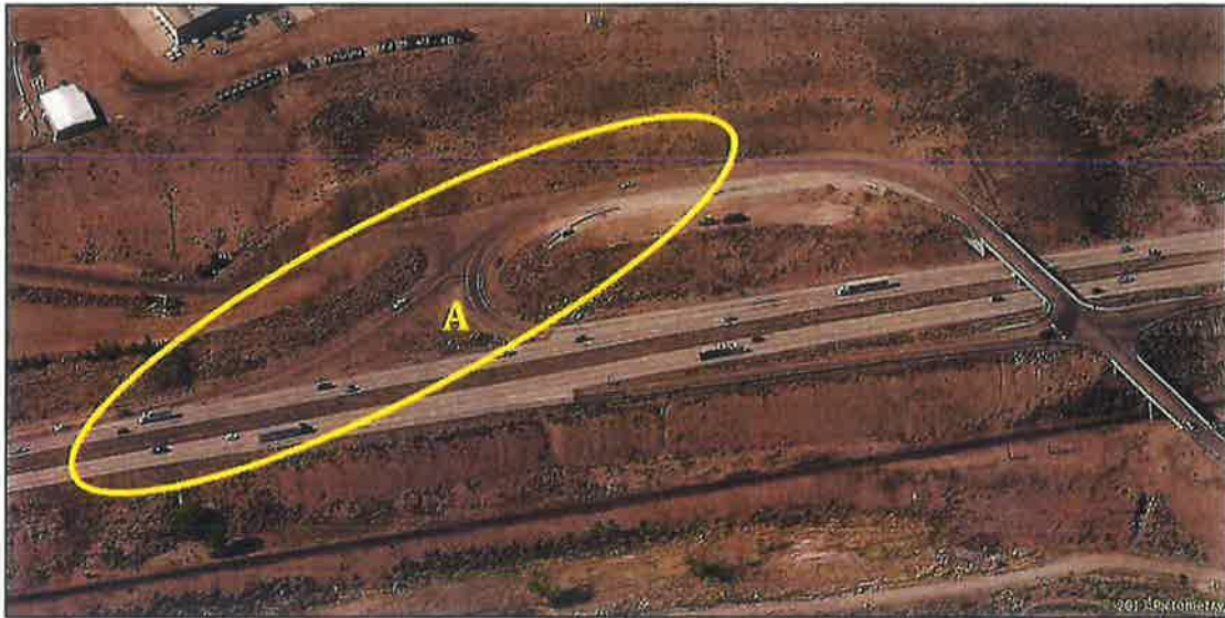
Figure 3.4-32: The images depict the existing infrastructure connecting Lockwood to Interstate 80. The image illustrates an on-ramp with substandard length for safe entry onto the interstate (A), and sharp and narrow curvature which inhibits safe two-way vehicle and truck travel (B). (Source: Storey County Planning Department, 2015)
